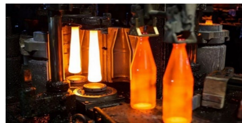
Figure 1 – Glass is glowing from heat during the blow-blow process.
