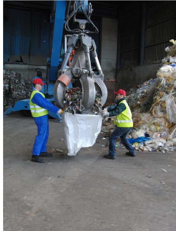
Figure 24: Obtaining a sample from the mixed plastics using an excavator.
