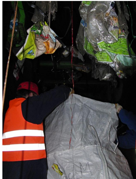
Figure 31: Obtaining a sample from the mixed plastics fraction in the bunker in Kempen.
