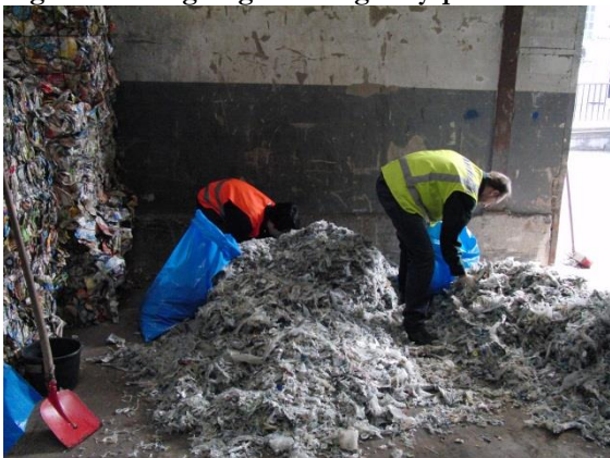
Figure 48: Obtaining grab samples to measure the dry matter of the light by-products.
