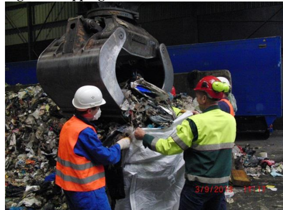
Figure 12 Obtaining a grab sample using the excavator
