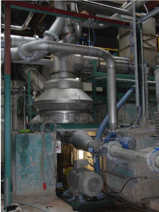
Figure 41: The Codukte recycler used to produce the fibre pulp.
