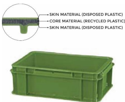
FIGURE 25: TRANSPORT CRATE WITH TWO DIFFERENT TYPES OF REUSED PLASTICS (SOURCE: SEKISUI CHEMICAL CO. LTD)
